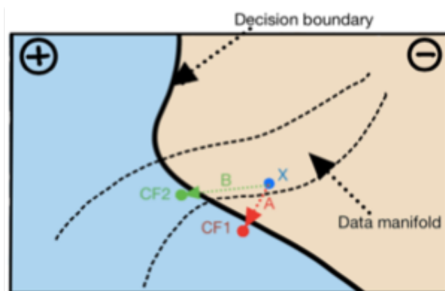
Figure 1: Two possible paths for a datapoint (shown in blue), originally classified in the negative class, to cross the decision boundary. The end points of both the paths (shown in red and green) are valid counterfactuals for the original point. Note that the red path is the shortest, whereas the green path adheres closely to the manifold of the training data, but is longer.
